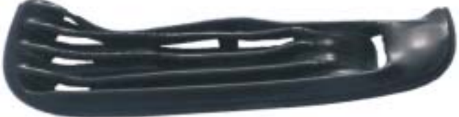
Original plastic panel distorted from heat and is no longer serviceable.
