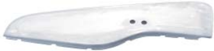
Original plastic panel distorted from heat and is no longer serviceable.
